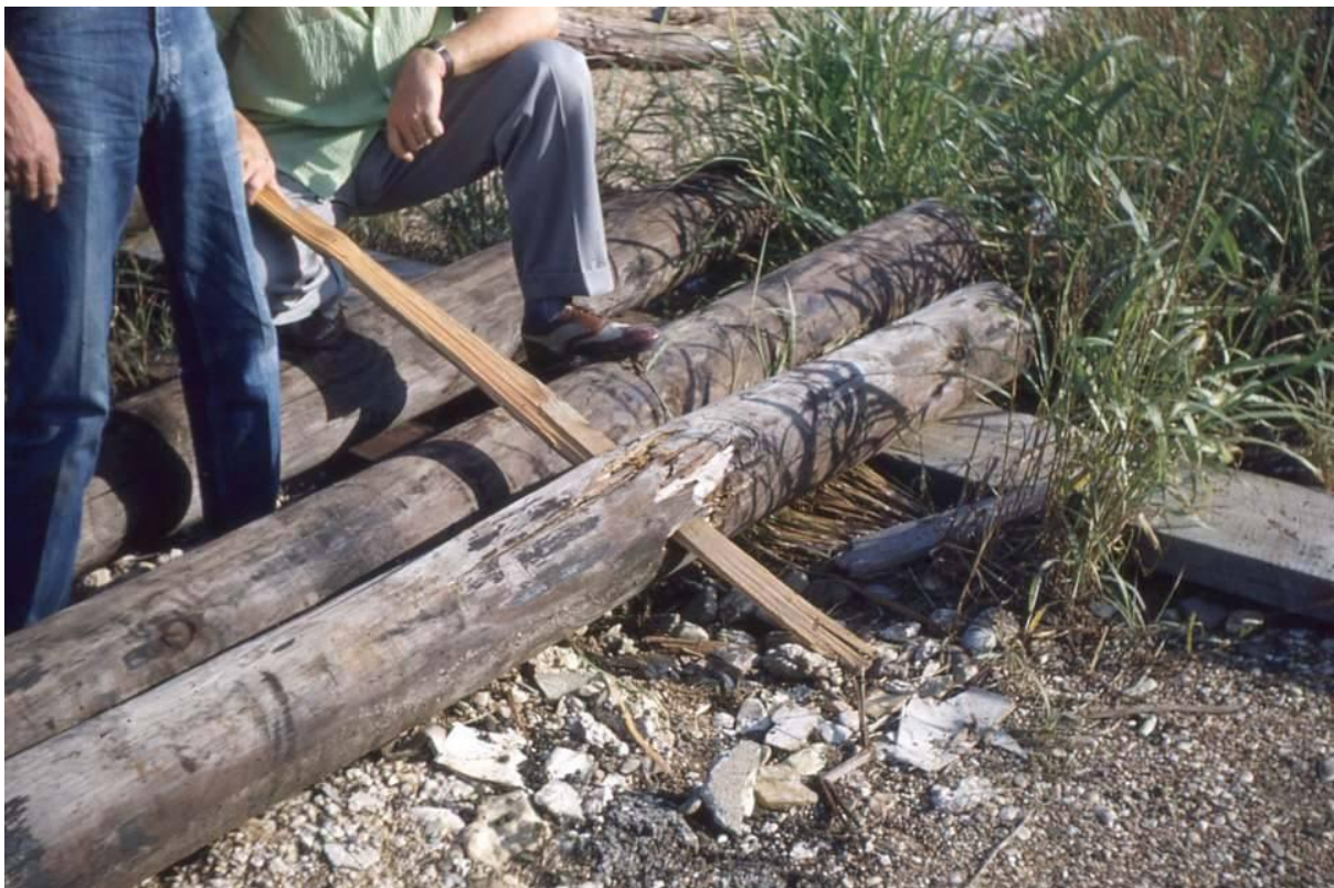
The force of the wind drove the smaller piece of wood through the pole!
